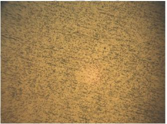
Figure 4: Micrograph of Al-12wt%Si + 0.08%S alloy casting (200x).
