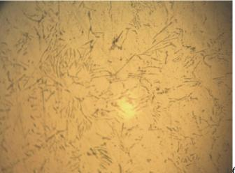
*Figure 1a: Micrograph of unmodified Al-12wt% S*<sub>1</sub>7 *alloy casting (200x).* 18
