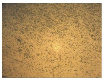
*Figure 5: Micrograph of Al-12wt%Si + 0.1% Si alloy casting (200x).*
