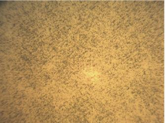
*Figure 3: Micrograph of Al-12wt%Si + 0.05%Salloy casting (200x).*
