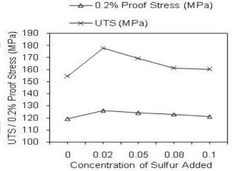
(% of the allov weight) Figure 6: Variation of UTS/0.2% Proof Stress of Al-*12wt%Si sand cast alloy with sulphur addition.*
