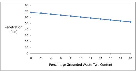
Figure 1: Penetration Test Values of Tyres Modified Bitumen
