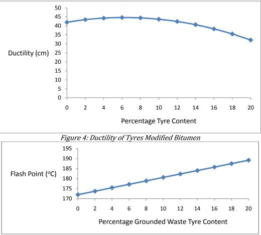
Figure 5: Flash Point of Tyres Modified Bitumen
