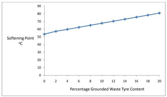
Figure 2: Softening Point of Tyres Modified Bitumen
