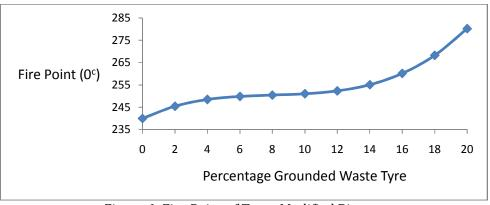
Figure 6: Fire Point of Tyres Modified Bitumen
