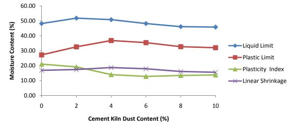
Figure 2: Variation of Atterberg Limits of Black Cotton Soil with Cement Kiln Dust Content
