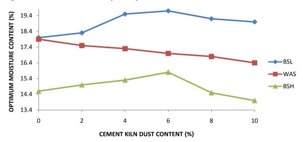
Figure 4: Variation of Optimum Moisture Content of Balck Cotton Soil with Cement Kiln Dust
