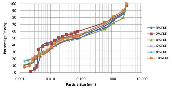
*Figure 1: Particle Size Distribution curves of combined Dry and Hydrometer Sedimentation Tests of Black Cotton Soil-Cement Kiln Dust Mixtures*
