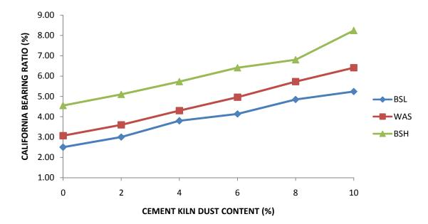
Figure 6: Variation of Soaked California Bearing Ratio of Black Cotton Soil with Cement Kiln Dust Content
