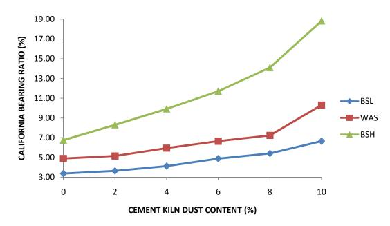
Figure 5: Variation of Unsoaked California Bearing Ratio of Black Cotton Soil with Cement Kiln Dust Content
