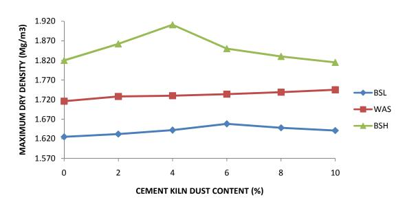
Figure 3: Variation of Maximum Dry Density of Black Cotton Soil with Cement Kiln Dust Content
