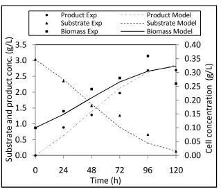
*Figure 2: Comparison between experimental and model predicted results for Haldane model*
