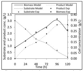
*Figure 4: Comparison between experimental and model predicted results for hyperbolic model*
