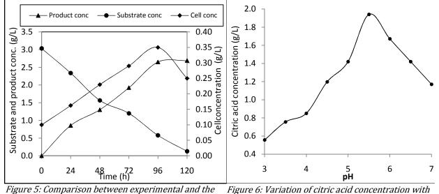
*Figure 5: Comparison between experimental and the model predicted results for hyperbolic model*
