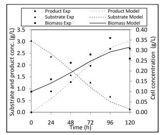
*Figure 1: Comparison between experimental and model predicted results for Monod model*
