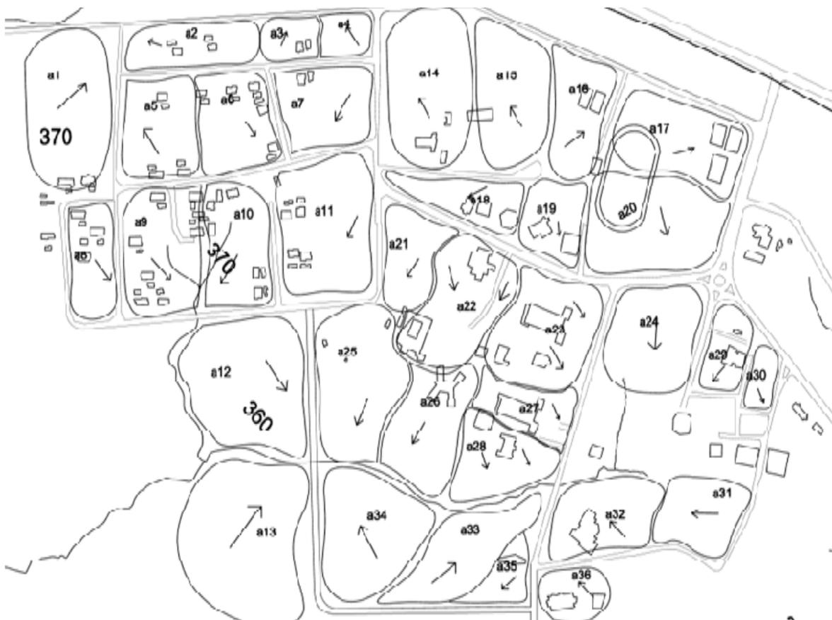
Figure 3: Layout of Stormwater Subcatchment Areas and the Proposed Stormwater Collection Networks
