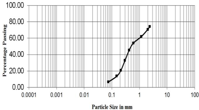
Figure 1a: Grading curve for fine aggregates
