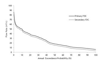
Figure 4: Primary and Secondary Flow Duration Curves for Opeki River
