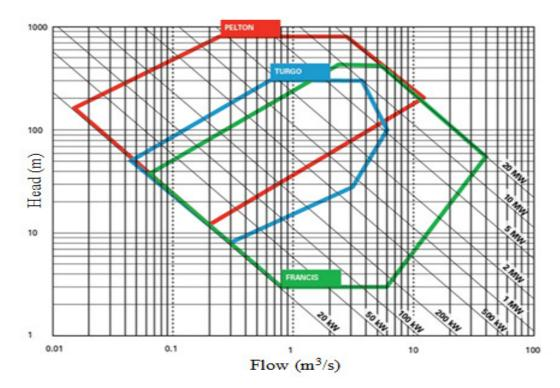
Figure 3: Turbine types and range of applications [17]
