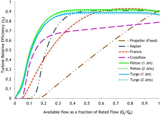
Figure 1. Turbine Efficiency Curves
