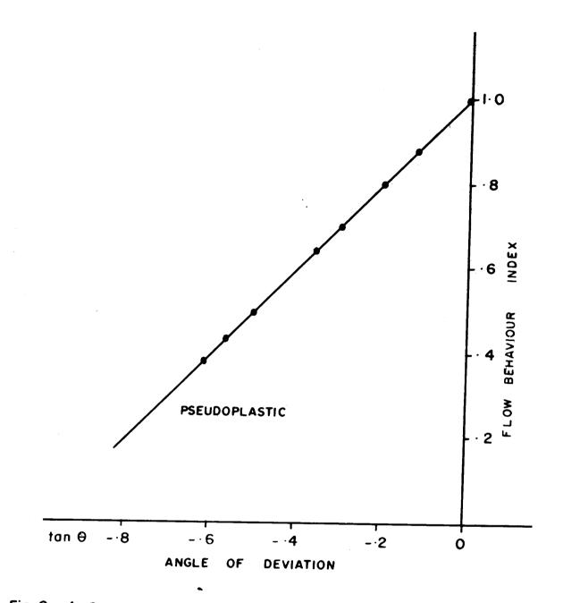
Fig. 8 A plot of flow behaviour index vs angle of deviation of pseudoplastic fluids.
