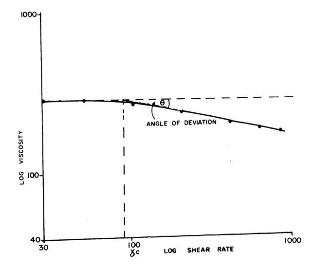
Fig 2 Flow behavior of a mixture of 80% corn syrup and 20% salad cream and angle of deviation from Newtonian flow
