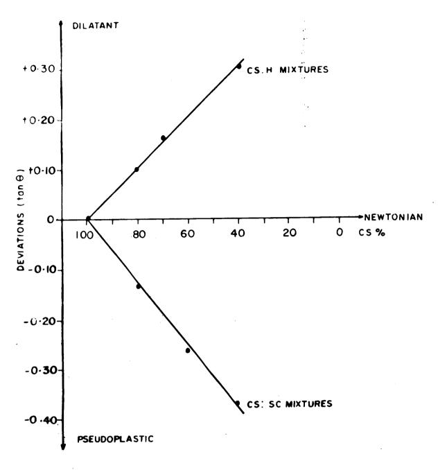
Fig. 9 Effects of mixing corm syrup (cs) with honey (H) and mixing salad cream (sc) with corn syrup on deviations from Newtonian flow.
