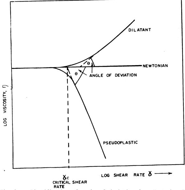
Fig. 1. Identification of angle of deviation from Newtonian Flow in Pseudoplastic and dilatants materials.
