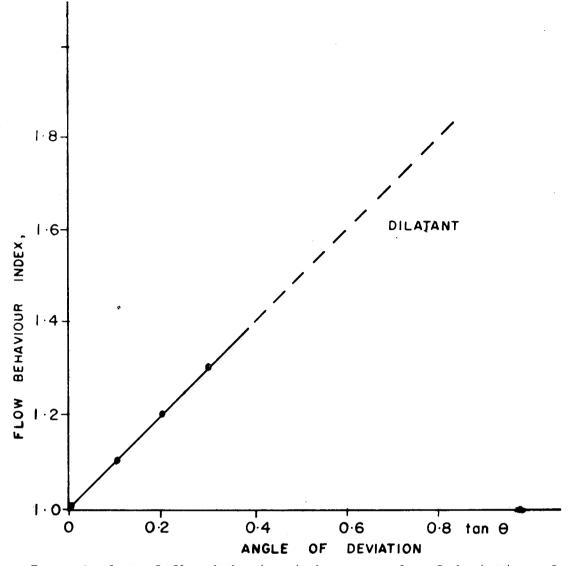
Fig. 7 A plot of flow behavior index vs angle of deviation of dilatants fluids.
