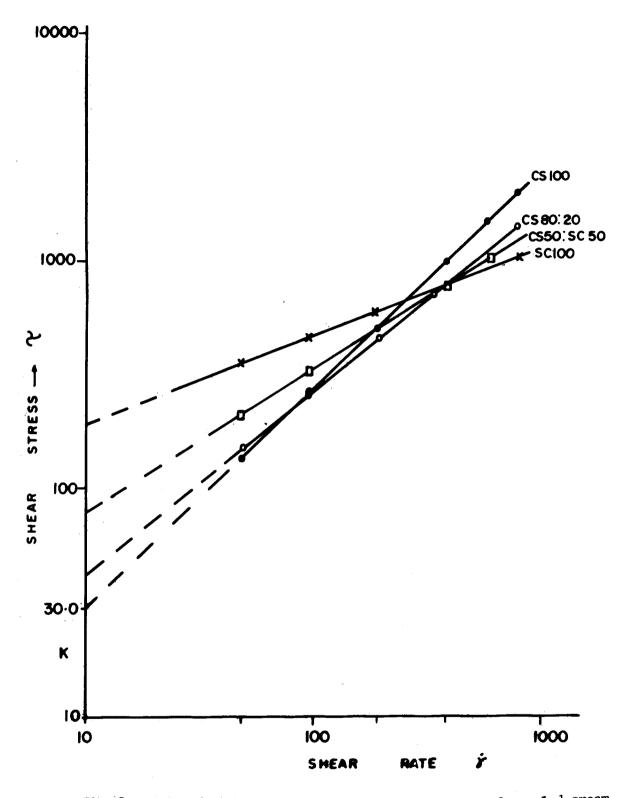
Fig. 6. Double log (shear stress vs shear rate) plots for salad cream (sc), corn syrup (cs) and mixtures of corn syrup and salad cream.
