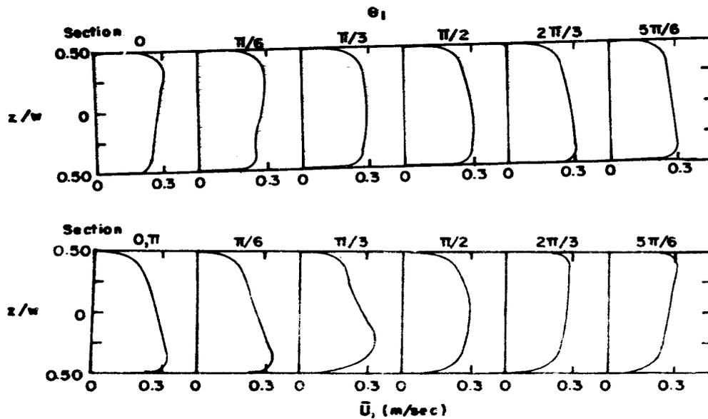
FIGURE 2. LATERAL DISTRIBUTION DEPTH-AVERAGED LONGITUDINAL VELOCITY. RUN 301/2/5
