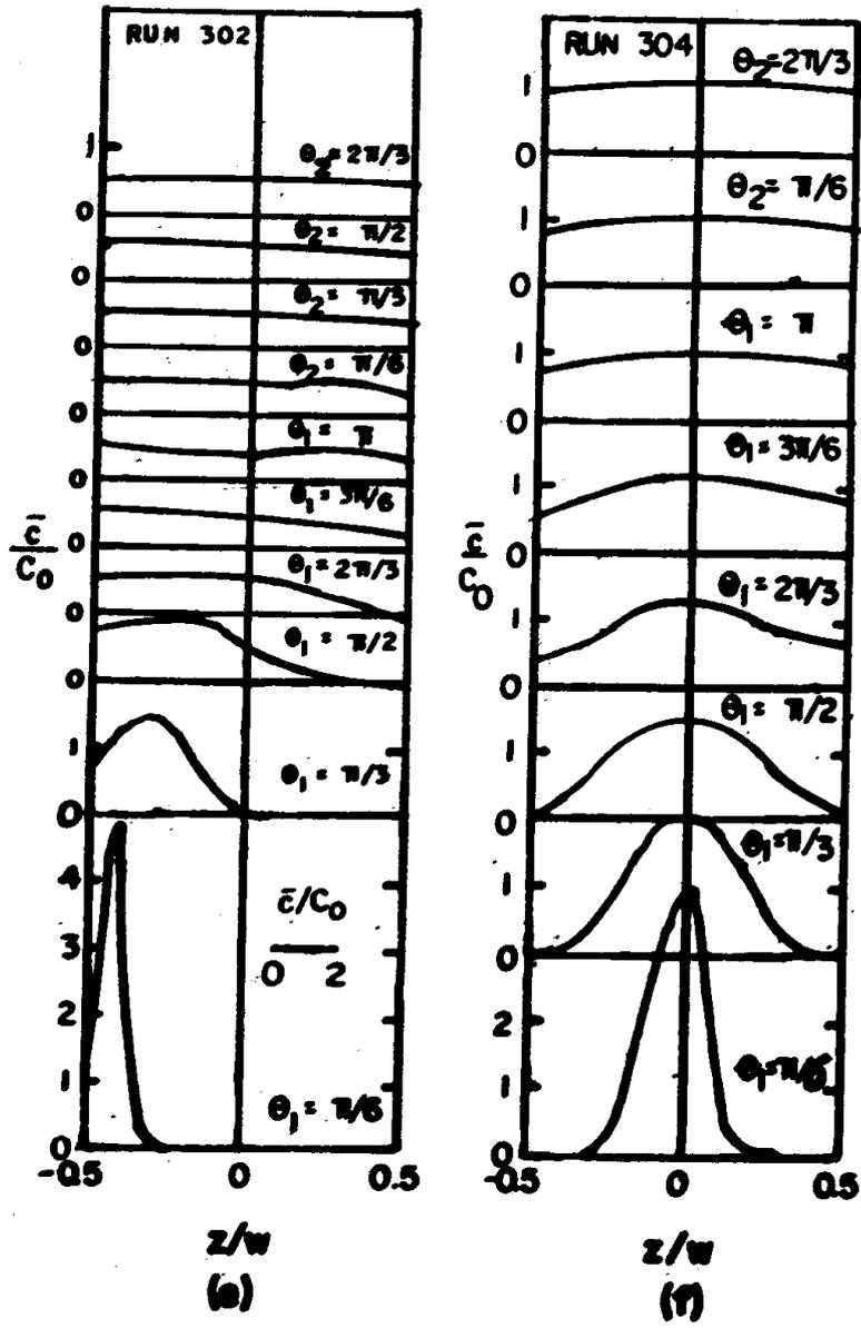
**FIGURE 5 TRANSVERSE DISTRIBUTIONS OF DEPTH-AVERAGED TRACER CONCENTRATION AT VARIOUS SECTIONS DOWNSTREAM OF SOURCE.**
