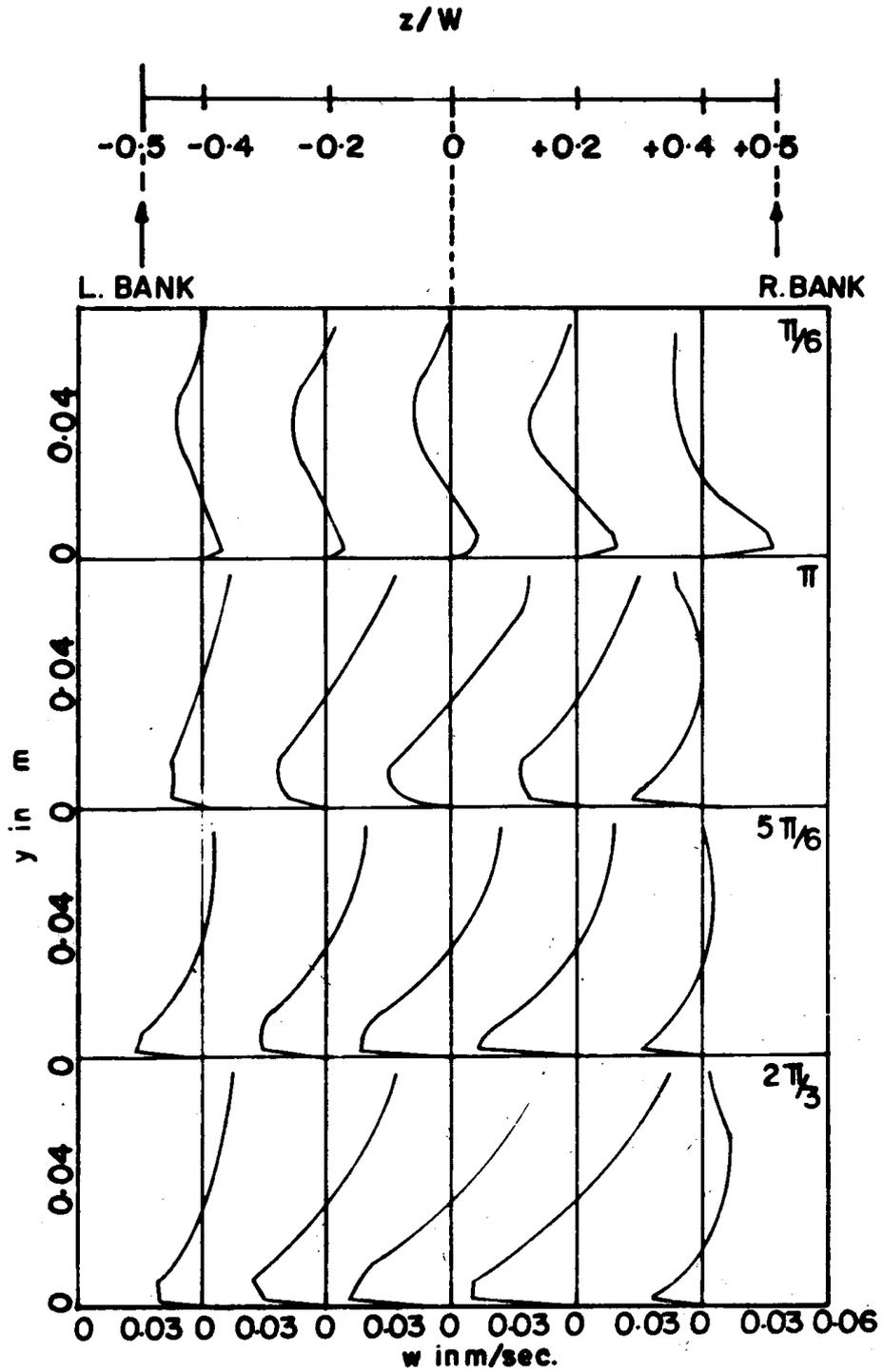
FIGURE 3b VERTICAL DISTRIBUTION OF TRANSVERSE VELOCITY. RUNS 301/2/3 SECTIONS  $\theta_1 = 2\pi/3$  TO  $\theta_2 = \pi/6$
