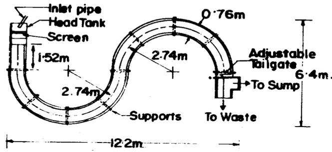
FIGURE 1A PLAN VIEW OF MEANDERING FLUME
