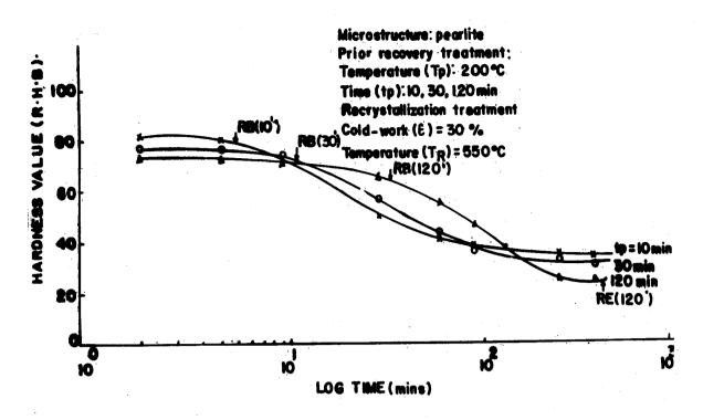
Figure 2. Variation of hardness with time during recrystallization annealing of a pearlitic microstructure after previous recovery heat-treatment for various times, tp.
