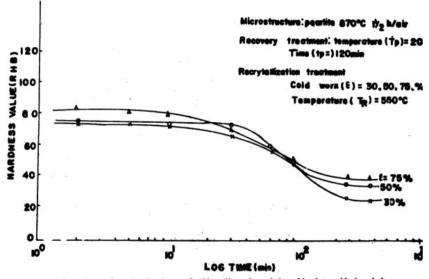
Figure 5. Effect of % Deformation (or degree of cold work) on the variation of hardness with time during recrystallization heat-treatment of a pearlitic microstructure after previous recovery heat-treatment (recovery time, t<sub>p</sub> maintained at 120 minutes in all cases.)
