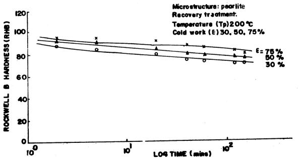
Figure 1. Variation of hardness with time during recovery heat-treatment of a specimen having a pearlitic
