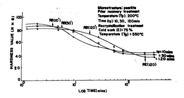
Figure 4. Variation of hardness with time during recrystallization annealing of a pearlitic microstructure after previous recovery heat-treatment for various times, tp. (% Deformation = 75; t<sub>p</sub> = 10min, 30min, 120min.)
