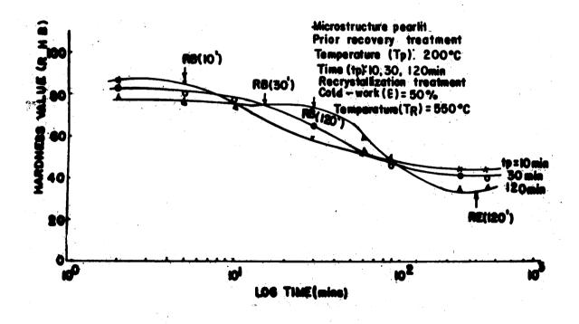
Figure 3. variation of hardness wan time during recrystallization annealing of a pearlitic microstructure after previous recovery heat-treatment for various times, tp. (% Deformation = 50; t<sub>p</sub> = 10min, 30min, 120min.)
