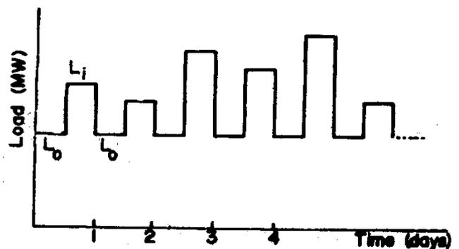
Figure 1: Sequence of loads used for load Model
