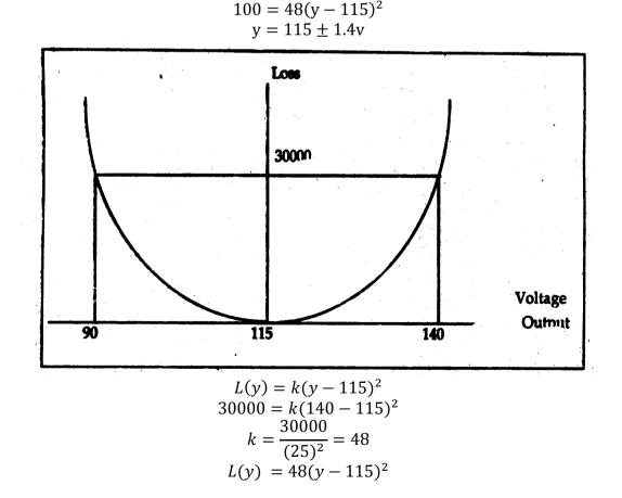
Figure 21: Obtaining the loss function
