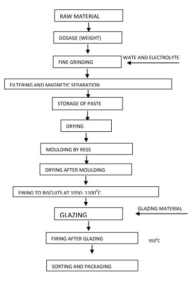
FIG.1 Flow diagram for tile production
