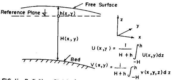
FIG. 1: Definition Sketch for the System of Equations (1)- (3).
