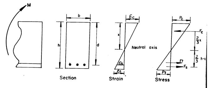
Figure I. Elastic Strain and Stress Blocks of Uncracked Reinforced Concrete Section
