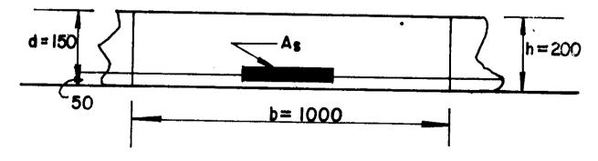
Figure 2. One Meter Length of the Section Under Design.
