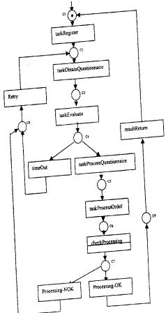
Fig. 3: A workflow process definition for epurchase
