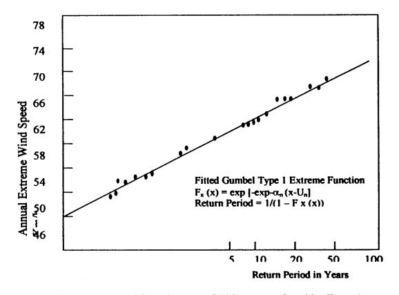
Fig. 2 Set of Annual Extreme Wind Speeds in NE-SW Direction fitted by Type 1 Asymptotic Extreme Value Distribution
