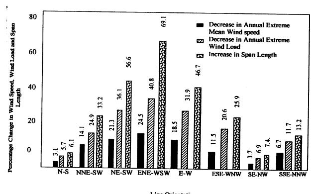
Line Orientation Fig. 7 Change in Annual Extreme Wind Speed, Wind Load, and Span Length for Different Line Orientations
