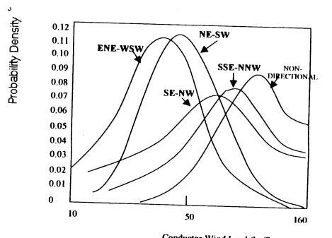
Conductor Wind Load (kg/Sq.m) Fig. 5 Probability Density Functions of the Extreme Wind Loads for Typical line Orientations
