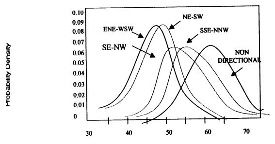
Extreme Mean Wind Speed (km/h) Fig.4 probability Density Functions of the Extreme Winds Speeds for typical line orientations
