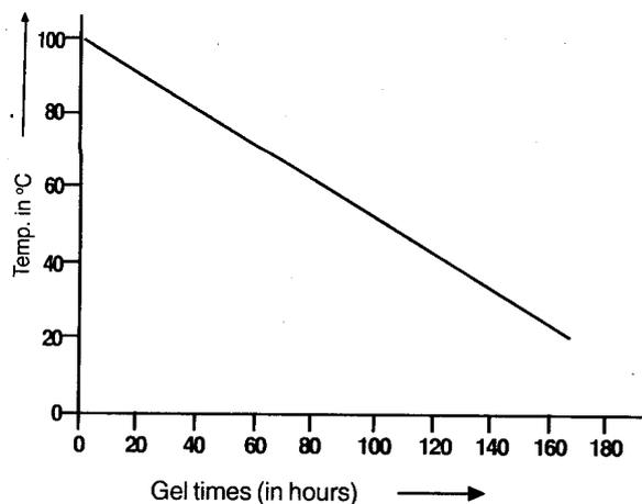
Fig. 3: Effect of Inhibitor, Catalyst and Temperature on gel times of (OCF 3-600) polyester resin.
