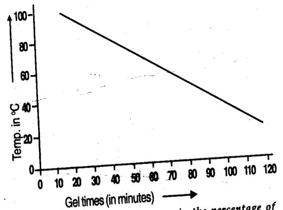
Fig. 6: Effect of further decrease in the percentage of accelerator added to composition in experiment 4.
