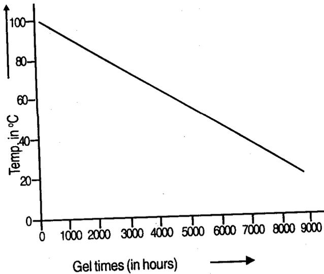
Fig. 2: Effect of Inhibitor and Temperature on gel times (OCF E-600) polyester resin.
