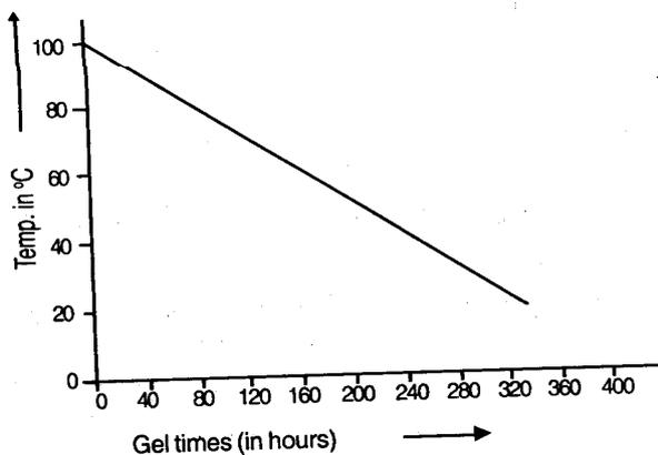
**Fig 1:** Effect of temperature only on gel times of (OCF E-600) polyester resin
