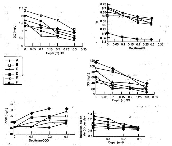
Fig.10: Variation on DO, PH, T, SS, COD and K with depth due to temperature differences (Day 6).
