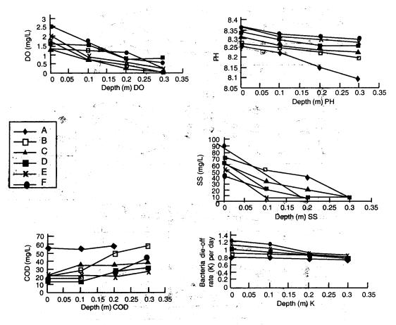
Fig. 5: Variation of DO, PH, T, SS, COD and K with depth due to temperature differences. (Day 1).
