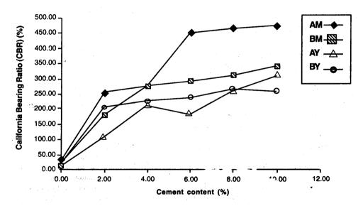
Fig. 4: Variation of California Bearing Ratio with Cement content.
