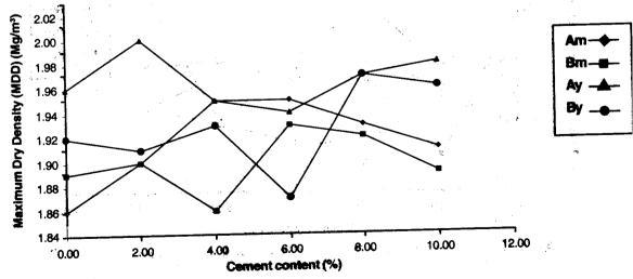
Fig. 1: Variation of Maximum Dry Density with Cement content
