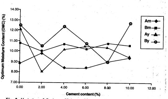
Fig. 2: Variation of Optimum Moisture Content with Cement content.
