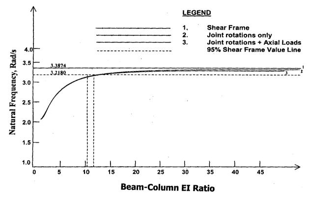
Ig4: Plot of Natural Frequency Against Beam-Column El Ratio for the 15-Storey Frame.
