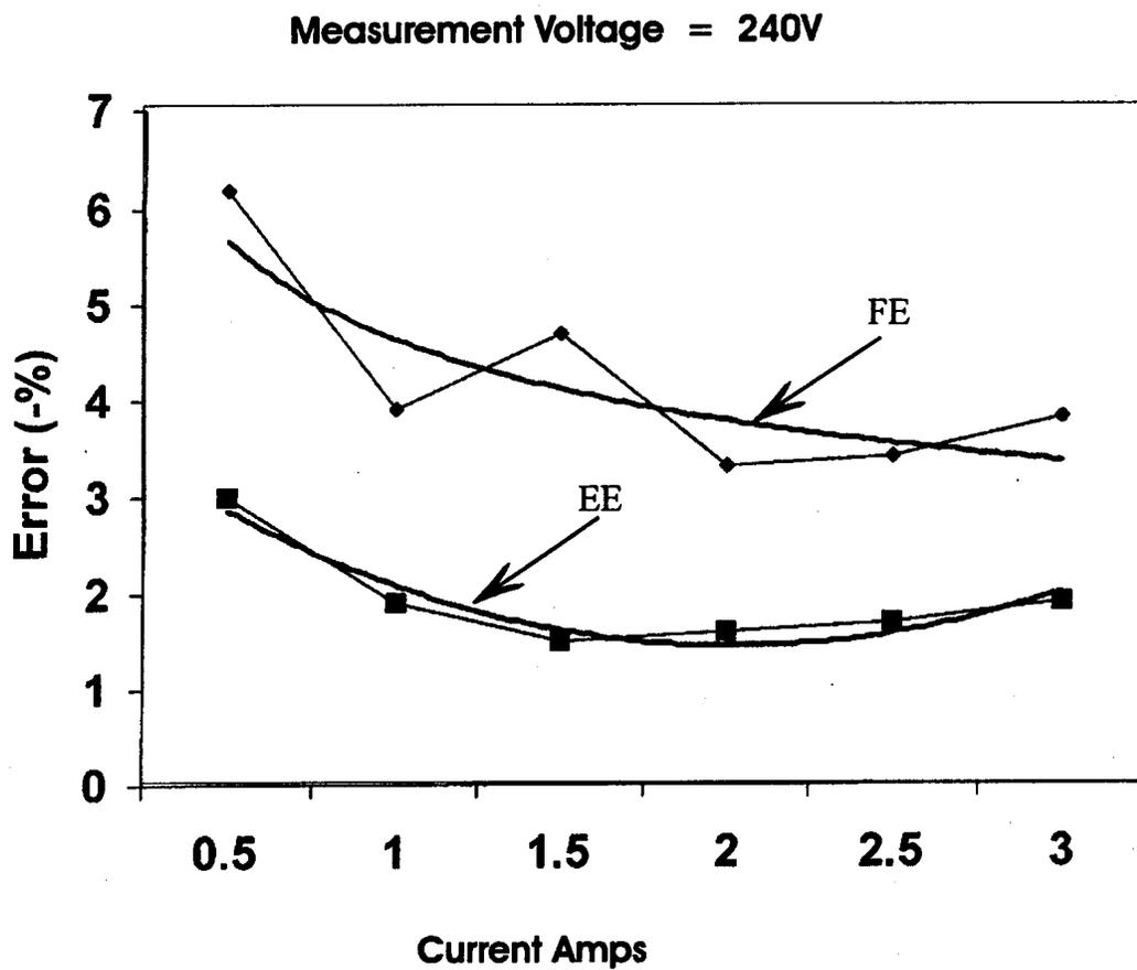
*Fig. 7: Errors of the Ferraris and the Electronic Meters.*
