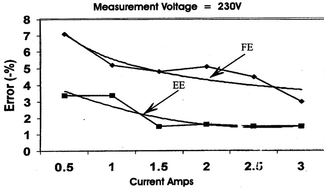
*Fig. 6: Errors of the Ferraris and the Electronic Meters.*
