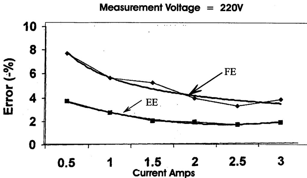
*Fig. 5: Errors of the Ferraris and the Electronic Meters.*
