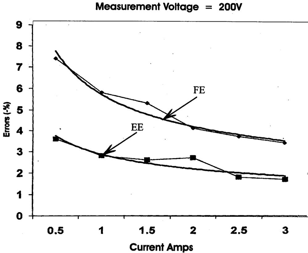
*Fig. 4: Errors of the Ferraris and the Electronic Meters.*
