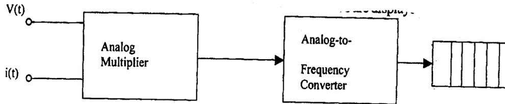
Fig. 1: Scheme for Electronic Energy meter Realization.
