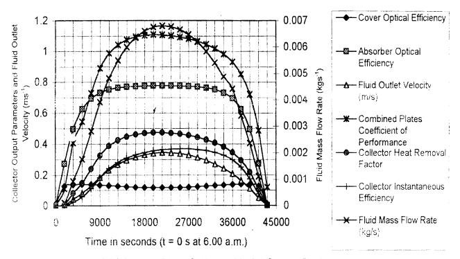
Fig. 3b. SSSCA Flat Plate Collector Model Output Performance Parameters and Fluid Mass Flow Rate and Outlet Velocity on 16-03-02
