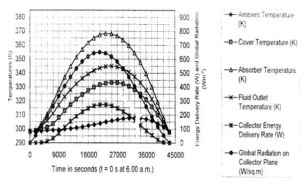
Fig. 3a SSSCA Flat Plate Collector Model Input and Output Parameters on 16-03-02  $T_a = T_f = 298.052408 + 2.262E-04t - 2.187E-08t^2 + 1.8432E-12t^3 - 3.385E-17t^4$  K, H = 16.4 MJm<sup>-2</sup>
