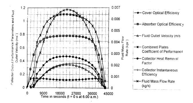
Fig. 2b SSSCA Flat Plate Collector Model Output Performance Parameters and Fluid Mass Flow Rate and Outlet Velocity on 14-03-02
