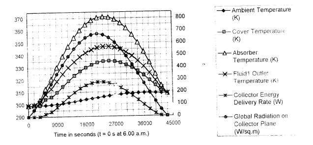
Fig 2a SSSCA Flat Plate Collector Model Input and Output Parameters on 14-03-02  $T_{d} = T_{fr} = 299.09883 - 1.323E-04t + 3.596E-08t^{2} - 8.711E-13t^{3} + 5.1751E-18t^{4}$  K, H = 17.0 MJm<sup>-2</sup>
