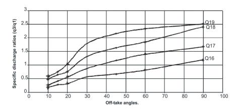
Fig. 2: Effect of off-take angles on specific discharge ratios for flows at concave channel bifurcation
