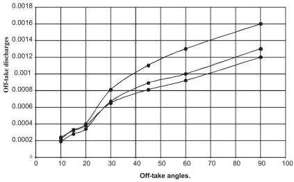
Fig.5: Plot of measured and predicted off-take discharges against off-take angles for Q18.
