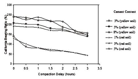
Figure 5: Variation of California Bearing Ratio with Compaction Delay for stabilized lateritic soils
