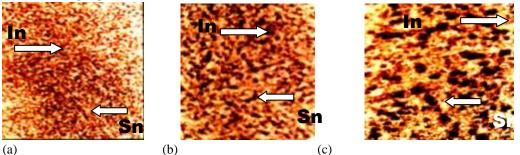
Fig.3 Microstructures of 58Sn-42In at different magnifications: (a) X50 (b) X100 (c) X200
