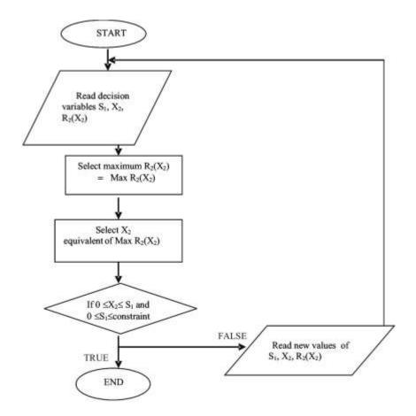
Fig 2: The Algorithm of the Stage 1 Flowchart of the TORA Software Dynamic Programming Calculations.
