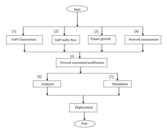
Figure 1: Flowchart Illustrating VoIP Deployment
