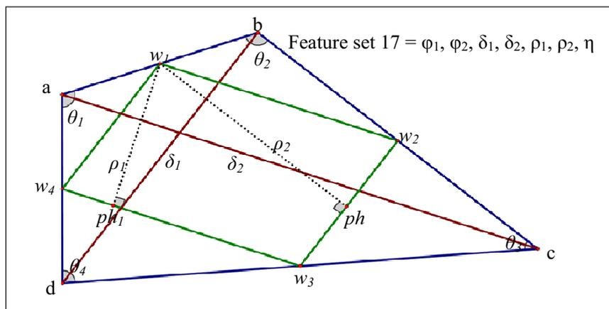
Figure 6: Feature set 17 comprising 7 features namely,  $\varphi_1, \varphi_2, \delta_1, \delta_2, \rho_1, \rho_2, \eta$ .
