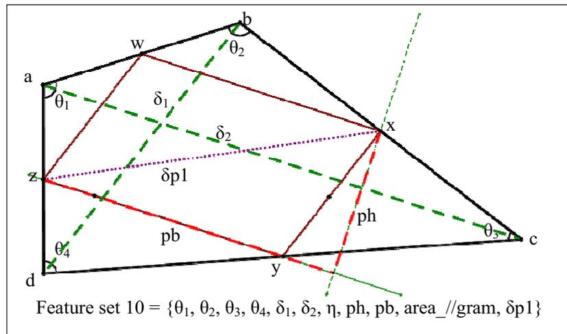
Figure 5: Feature set 10 comprising 11 features namely,  $\theta_1, \theta_2, \theta_3, \theta_4, \delta_1, \delta_2, \eta, ph, pb, area\_//gram, \delta p1$ .
