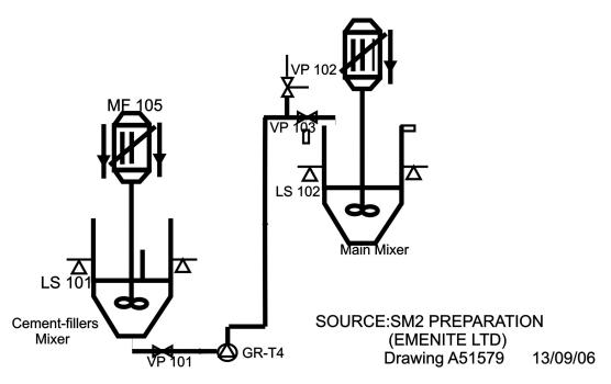
Figure 4: Sketch showing centrifugal pump GR-T4.
