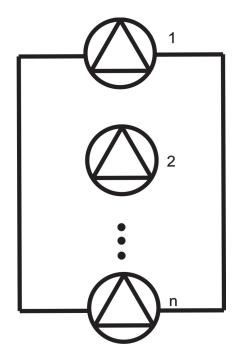
Figure 2: Reliability diagram for centrifugal pumps in parallel.
