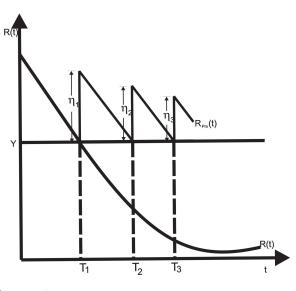
Figure 3: Effect of preventive maintenance on centrifugal pumps
