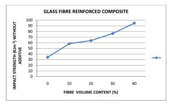
Figure 10: Graph of Impact Strength against Fibre volume content for Glass fibre reinforced composite without additives.
