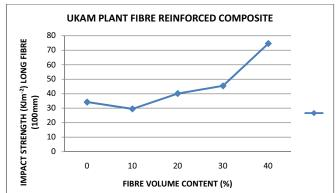
Figure 12: Graph of Impact Strength against Fibre volume content for Long Ukam plant fibre reinforced composite.
