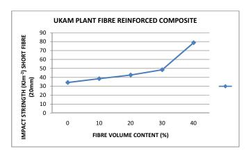
Figure 11: Graph of Impact Strength against Fibre volume content for Short Ukam plant fibre reinforced composite.
