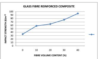
Figure 6: Graph of Impact Strength against Fibre volume content for a Glass fibre reinforced composite.
