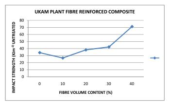
Figure 5: Graph of Impact Strength against Fibre volume content for an untreated Ukam plant fibre reinforced composite.
