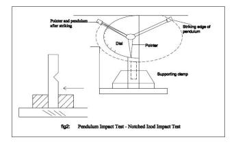
Figure 2: Pendulum Impact Test – Notched Izod Impact Test.
