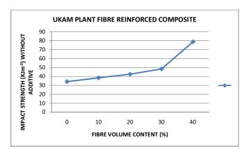
Figure 8: Graph of Impact Strength against Fibre volume content for Ukam plant fibre reinforced composite without additives.
