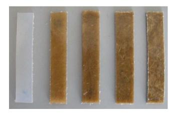
Figure 1: Impact testing specimens of Ukam plant fibre reinforced specimens.
