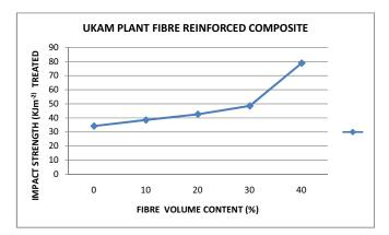
Figure 4: Graph of Impact Strength against Fibre volume content for a treated Ukam plant fibre reinforced composite.
