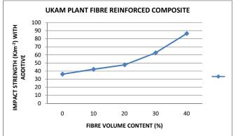
Figure 7: Graph of Impact Strength against Fibre volume content for Ukam plant fibre reinforced composite with additives.
