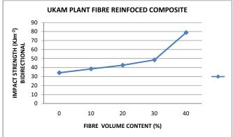
Figure 13: Graph of Impact Strength against Fibre volume content for a bi-directional Ukam plant fibre reinforced composite.
