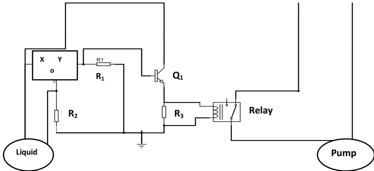
Figure 4: Circuit diagram of the water level controller.
