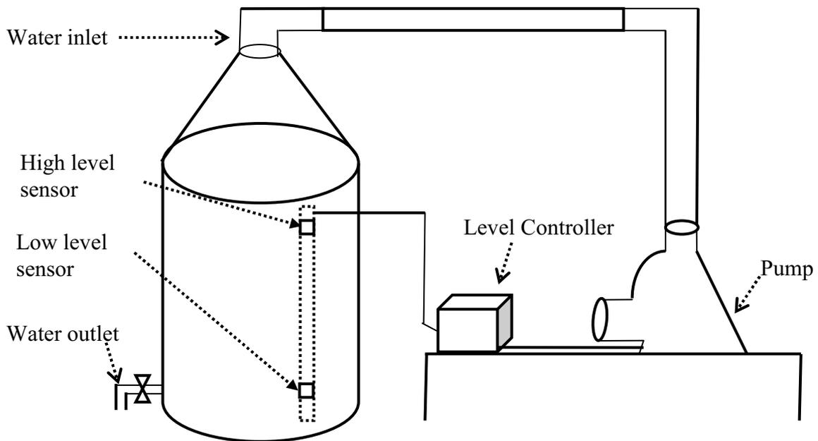
Figure 1: Schematic of the tank and regulator.
