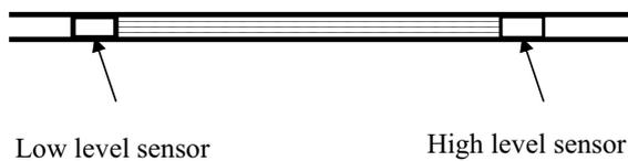
Figure 2: Schematic of the Sensor Assembly.
