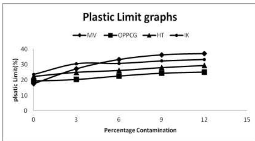
Fig 3: Graph of plastic limit vs percentage contamination
