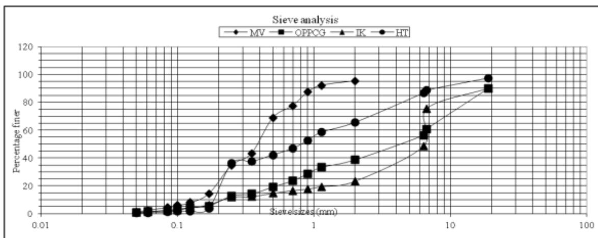
Fig 1: Sieve analysis of the soil samples
