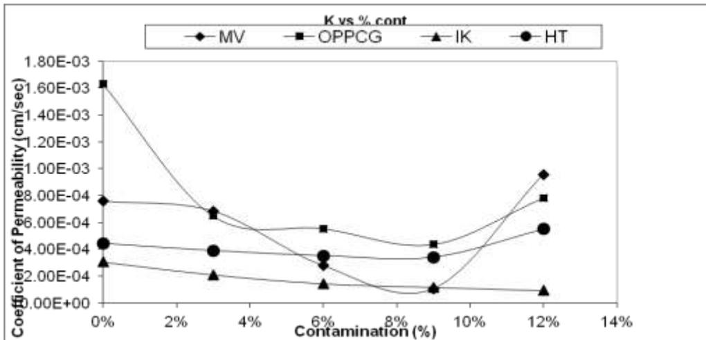
Fig 6: Graph of Coefficient of Permeability vs. Percentage contamination
