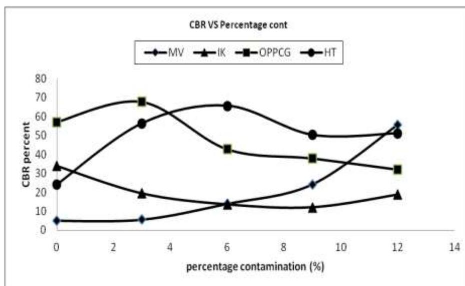
Fig 9: Graph of CBR vs. Percentage Contamination
