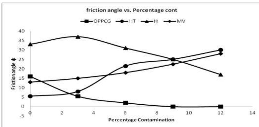
Fig 8: Graph of Friction angle vs. Percentage contamination
