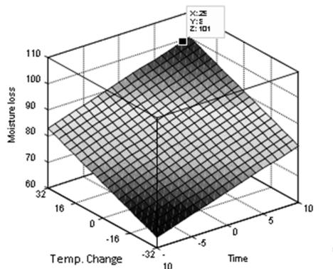
Figure 5: Surface plots showing the effect of temperature and time on the drying of sample C of cocoa beans
