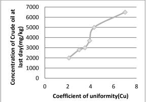
*Figure2B: Concentration of Remaining Crude Oil (mg/kg) at last Day Vs Cu for very fine to coarse sand(Y)*
