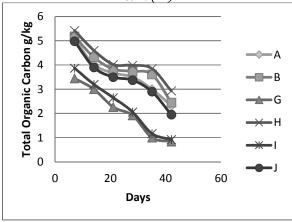
*Fig.6A: Total organic carbon Vs days for fine to coarse sand(X)*
