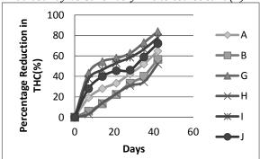
*Figure3A: Rate of Hydrocarbon Loss (% Reduction Vs Days for fine to coarse sand(X)*
