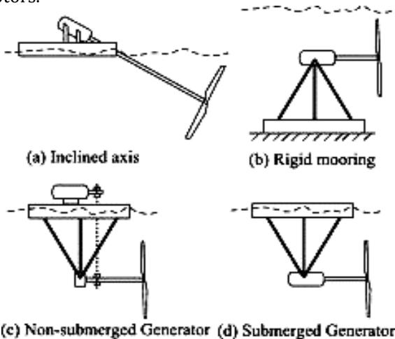
Figure 3: Axial (horizontal axis) hydrokinetic rotors (Source: [10]).
