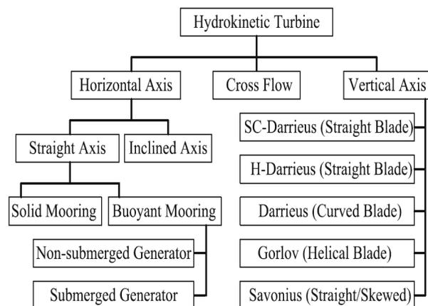
Figure 2: Classification of hydrokinetic turbines (Source: [8]).
