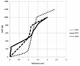
*Figure 2: Test results summary for masonry beam samples strengthened with DFRCC strips of 3cm.*
