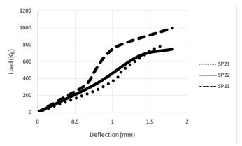
Figure 1: Test results summary for masonry beams strengthened with ECC strip of 2cm thickness.
