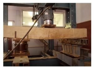
*Plate 1: Typical four-point loading set up for the tested samples (control and strengthened)*
