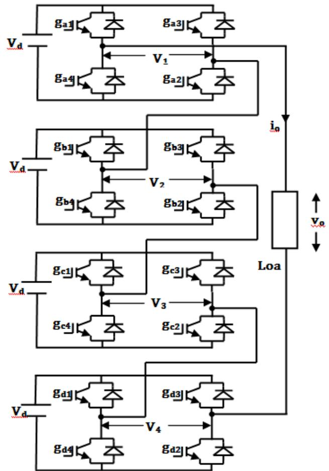
Figure 1: Configuration of 9-level cascade H-bridge multilevel inverter.
