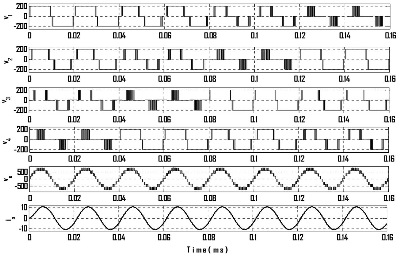
Figure 6: Simulated output voltages and load current
