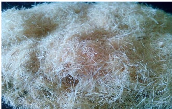
Figure 1: Chopped and treated Sisal Fibers
