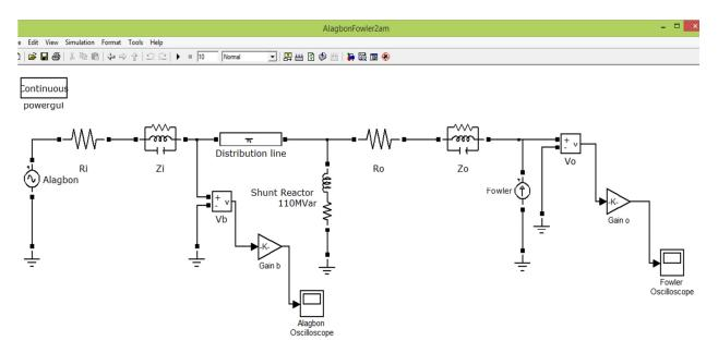
Figure 2: Formulated Model of Distribution Line Alagbon – Fowler Busbars as example
