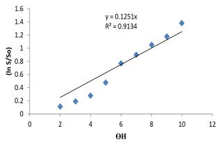
Figure 3: Determination of kinetic constant for first order model
