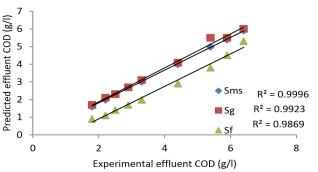
Effluent substrate for Modified Stover-Kicannon Model (SMs) R<sup>2</sup>=0.9996, Grau Second Order Model (Sg) R<sup>2</sup>=0.9923, First Order Model (Sf) **R<sup>2</sup>=0.9869**
