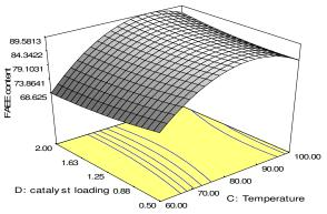
*Figure 4: Profile of response surface of biodiesel yield with catalyst loading and Temperature*
