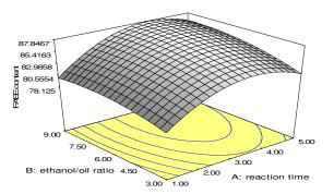
*Figure 2: Profile of response surface of biodiesel yield with ethanol/oil molar ratio and reaction time*
