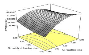
*Figure 1: Profile of response surface of biodiesel yield with catalyst loading and reaction time*
