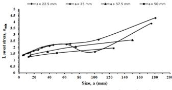
*Fig 8: Lowest stress against size, a for the end-web to centre-web of 1:2*
