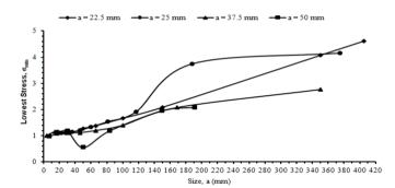
*Fig. 7 Lowest stress against size, a for the end-web to centre-web ratio is 1:1*
