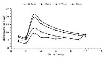
*Fig. 2: Maximum stress against the number of cavity for the end- web to centre ratio of 1:1*
