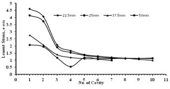
*Fig. 4: Lowest Stress against number of cavity for the end-web to centre-web ratio of 1:1*
