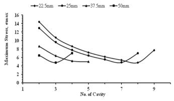
*Fig. 1: Maximum stress, σ max against the number of cavity where end-web to centre web ratio is 1:2*
