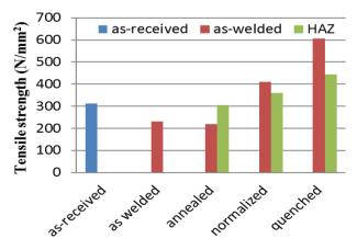
Fig. 2: Effect of post- weld heat treatment on the tensile strength of arc- welded medium carbon steel samples
