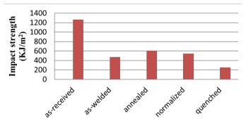
*Fig. 5: Effect of post- weld heat treatment on the Impact strength of arc- welded medium carbon steel samples*
