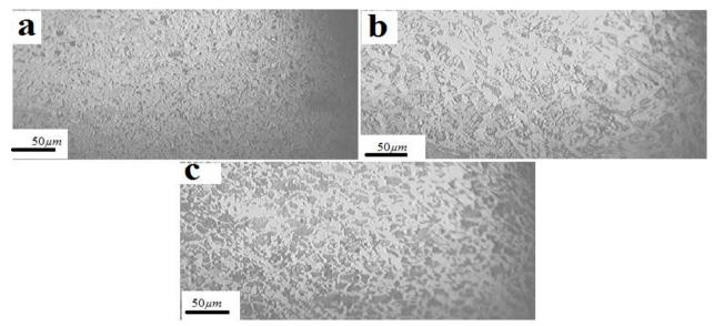
**PLATE 1:** optical micrograph of (a) as-received medium carbon steel, the structure show pearlite (dark patches) in ferrite matrix (white patches). (b) as-welded weldment, this structure shows as-cast structure of coarse pearlite (dark patches) in ferrite matrix (white patches). (c) as-welded Heat Affected Zone (HAZ), the structure shows coarse pearlite (dark patches) in ferrite matrix (white patches). Etchant: 2% Nital, (x200).
