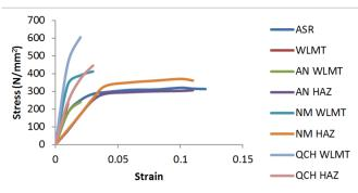
LEGEND: ASR: As-received, WLMT: Weldment, AN: Annealed, NM: Normalized, QCH: Quenched, HAZ: Heat affected zone
