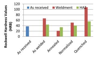
*Fig. 4: Effect of post- weld heat treatment on the Hardness profiles of arc- welded medium carbon steel samples*
