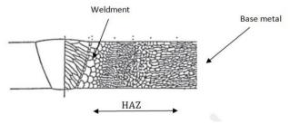
*Fig. 1: Schematic illustrations of single V-groove butt joint, showing various zones on the work piece (Source: Merchant, 2015)*
