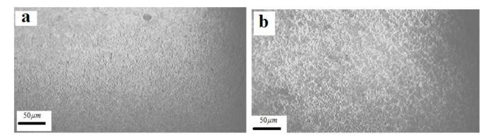
PLATE 3: optical micrograph of (a) quenched weldment sample, the structure shows martensite. (b) Quenched HAZ sample, the structure shows fine grains of equiaxed pearlite in ferrite matrix. Etchant: 2% Nital, (x200).
