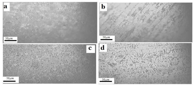
**PLATE 2:** optical micrograph of (a) annealed weldment sample, this structure shows coarse pearlite and ferrite. (b) annealed (HAZ) sample, this structure shows coarse pearlite in large proportion of ferrite (c) of normalized weldment sample, the structure shows refined grains of pearlite in ferrite matrix. (d) normalized HAZ sample, the structure shows more refined grains of pearlite and ferrite structure. Etchant: 2% Nital.
