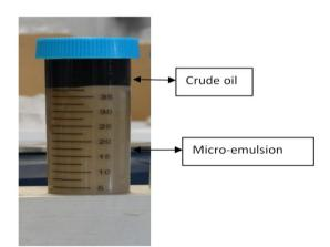
*Fig2: Centrifugation of oil-in-water emulsion sample. Time 2hrs, Speed 750rpm and Temp 250C (0.01mol + 0.100g solid).*
