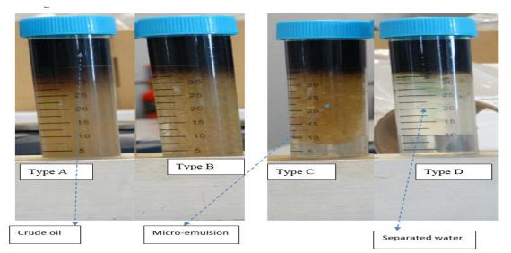
Fig 1: Centrifugation of oil-in-water emulsion samples. Time 2hrs, Speed 750rph, Temp  $25^{\circ}C.(A = 1.0 \text{ mol/L}, B = 0.05 \text{ mol/L}, C = 0.03 \text{ mol/L} and D = 0.01 \text{ mol/L}).$
