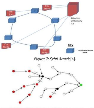
○ Sensor Node ● Base Station/Sink ● Attacker Node ● Affected Node → Subverted Link Figure 3: Blackhole Attack [8]
