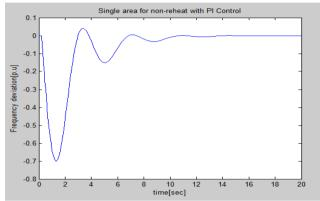
*Fig. 7: Frequency step response for a single area with PI control*
