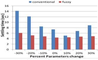
Fig. 13: Settling time under parameter variations.
