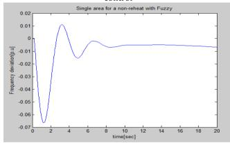
Fig. 8: Frequency step response for a single area with Fuzzy
