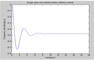
*Fig. 6: Frequency step response for a single area without control*
