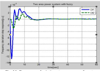
*Fig. 11: Frequency deviation step response for a two areas with Fizzy control*
