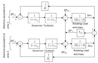
*Fig. 3: Two-area system without control for a non-reheat turbine*
