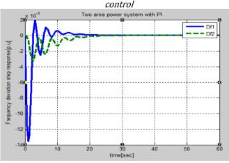
*Fig. 10: Frequency deviation step response for a two areas with PI control*
