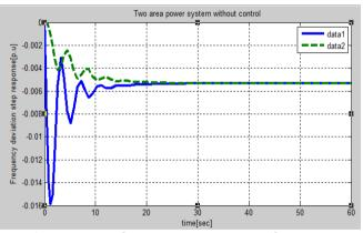
*Fig.9: Frequency deviation step response for two areas without control*
