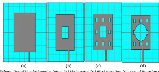
*Figure 2: Schematics of the designed antenna (a) Main patch (b) First iteration (c) second iteration (d) modified second iteration*
