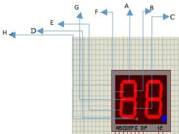
Fig. 2: Double Seven-Segment Display Unit with the 8<sup>th</sup> LED
