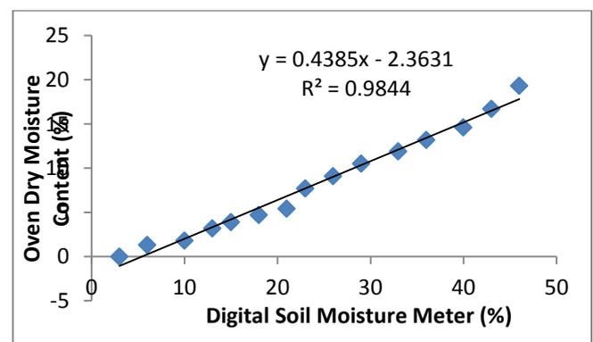
*Fig. 5: Calibration Graph for the Digital Soil Moisture Meter*
