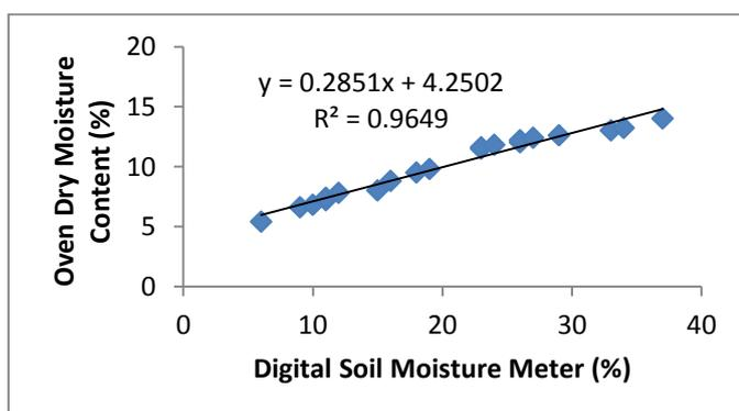
*Fig. 6: Validation Graph for Digital Soil Moisture Meter*
