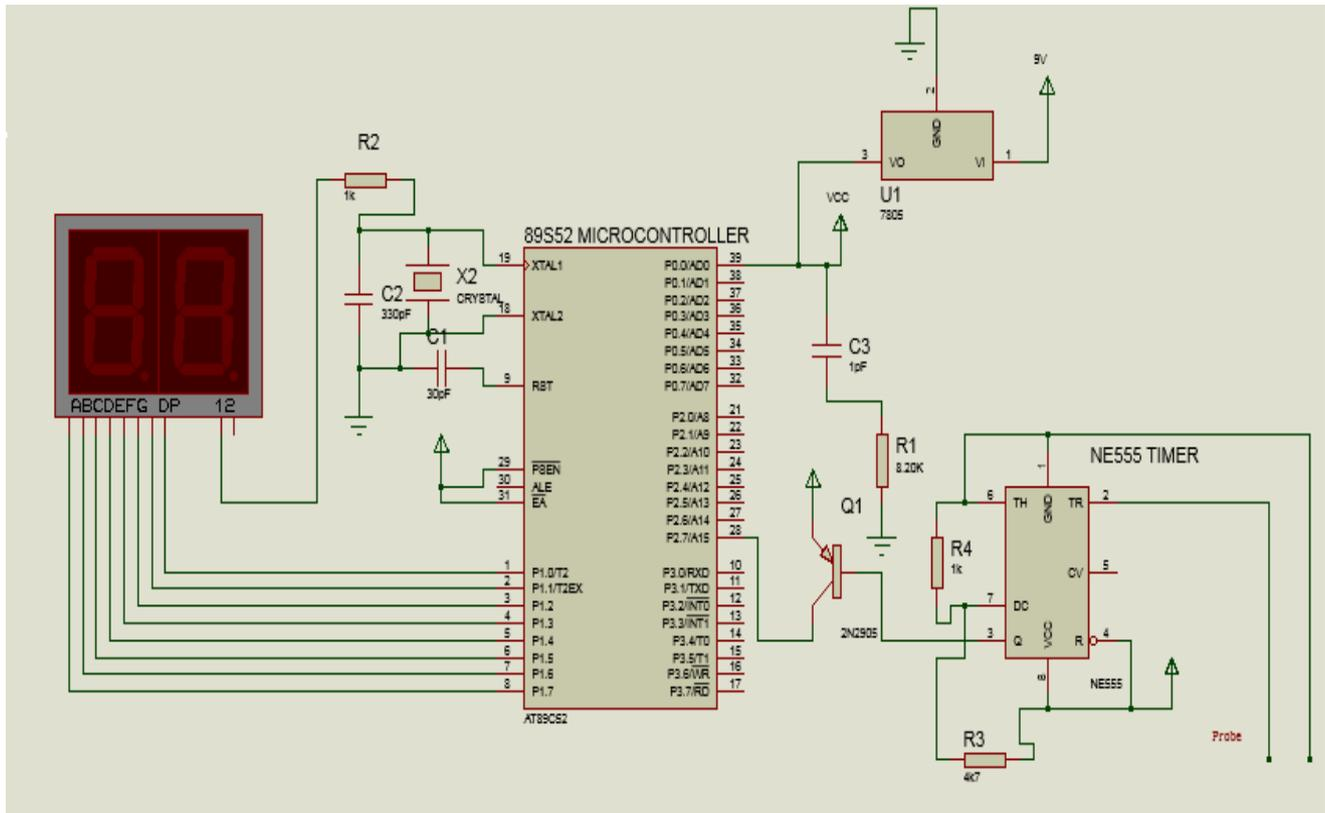
Fig. 3: Circuit Diagram of the Digital Soil Moisture Meter.
