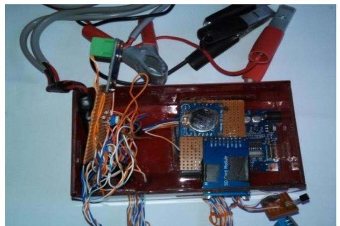
Fig. 3: Developed PV Monitoring System Prototype
